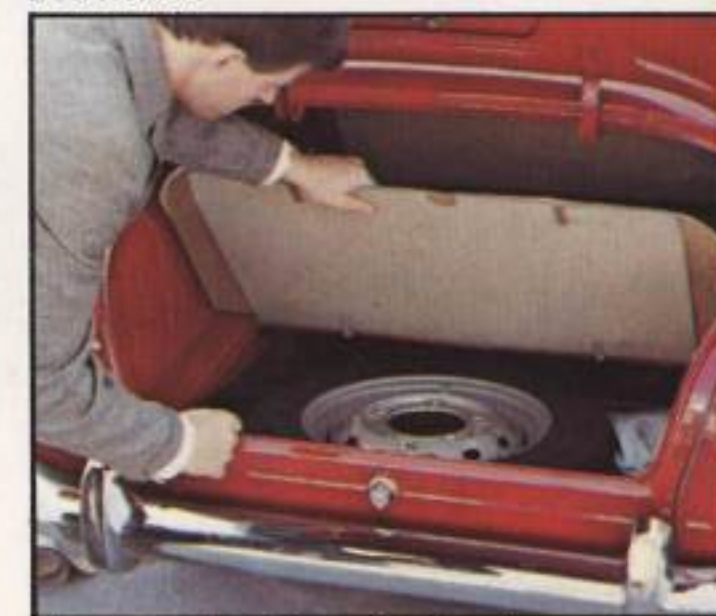
Spare wheel and tire in separate compartment.
