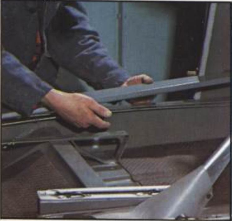
Brake lines are encased within steelplate.
