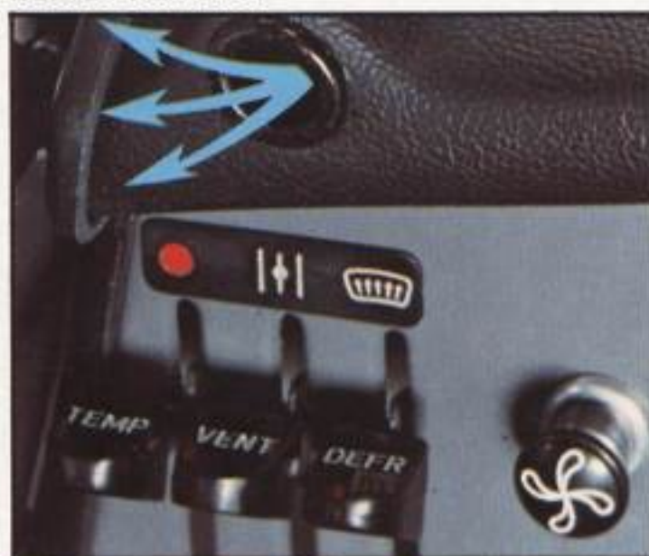
Ventilation and heating control levers.
