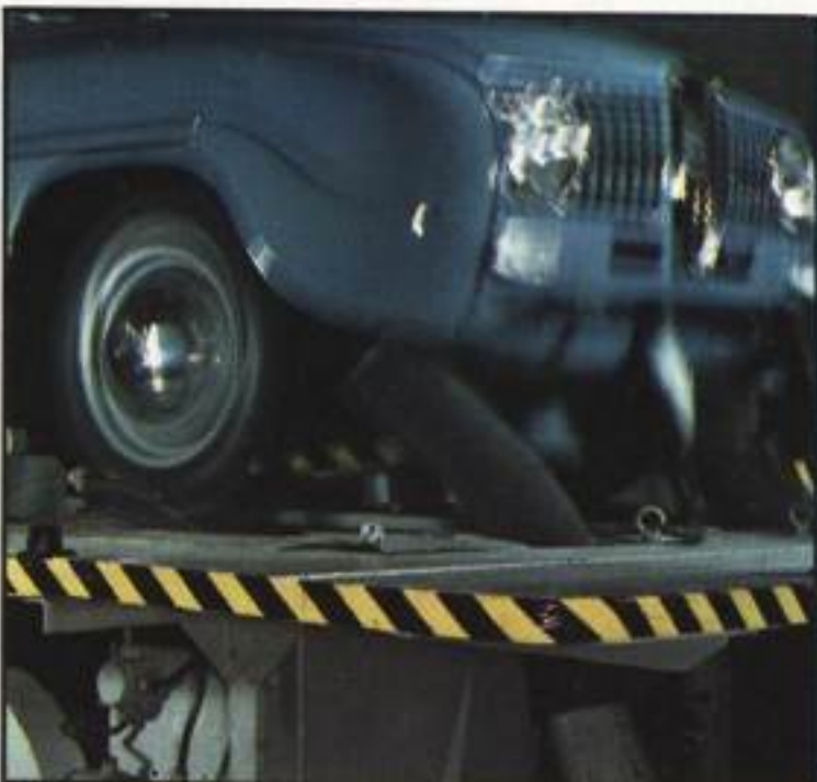
Torture testing on shaking machine.
