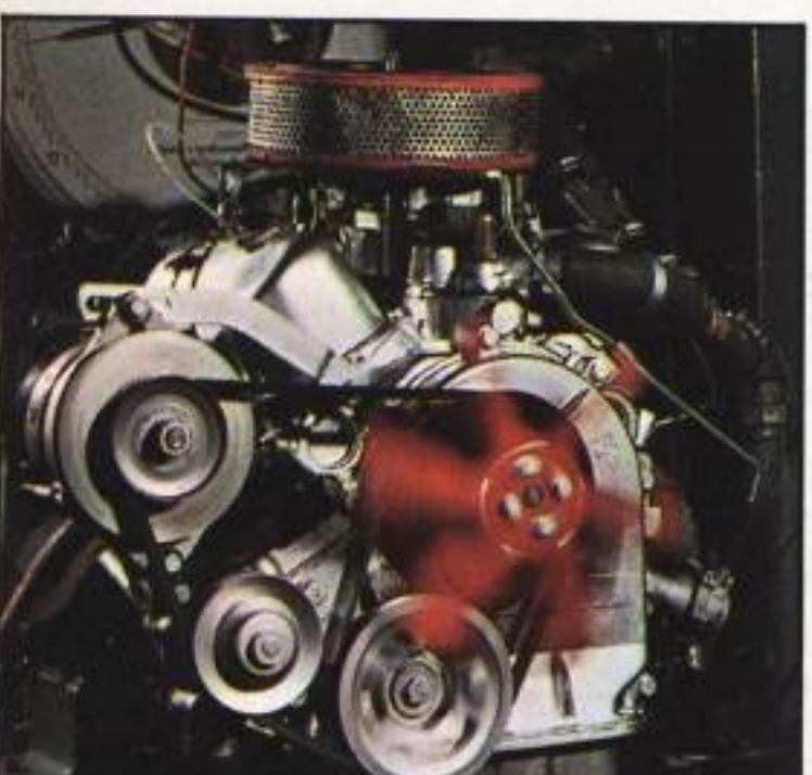
V4 engine during long-run test.
