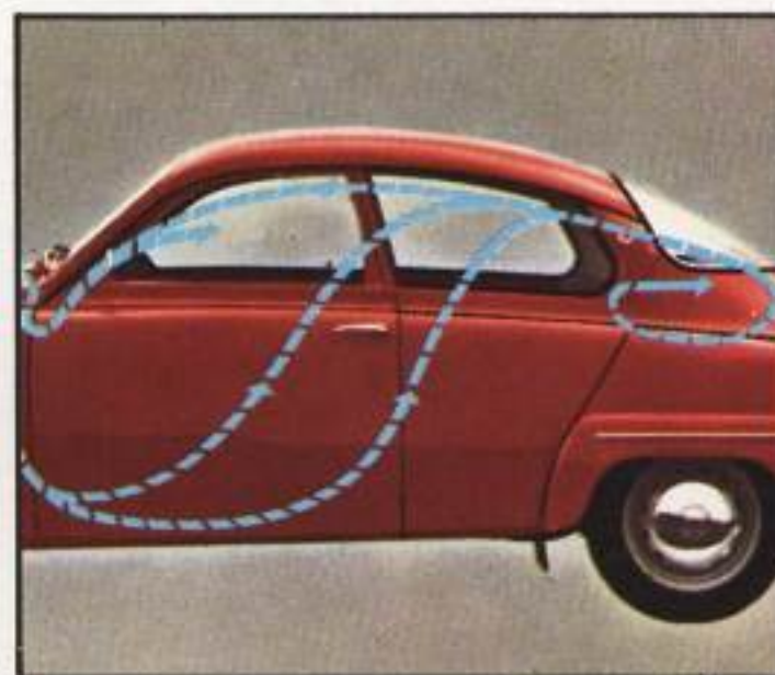
Air circulated through car and out rear.
