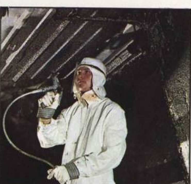
Body undercoated during manufacture.
